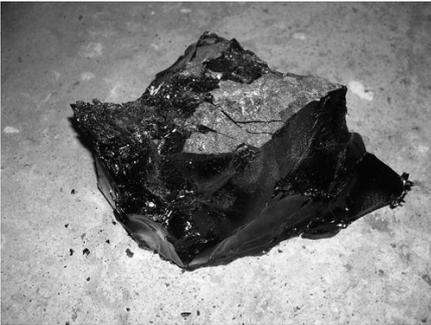
Bitumen is actually the liquid binder that holds asphalt together. The term bitumen is often mistakenly used to describe asphalt.
